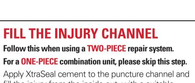
fill the injury from the inside out, with a suitable vulcanizing rubber stem. Then cut the stem 2/32 above the liner surface. The stem will then vulcanize to the injury channel and the repair unit, to prevent
